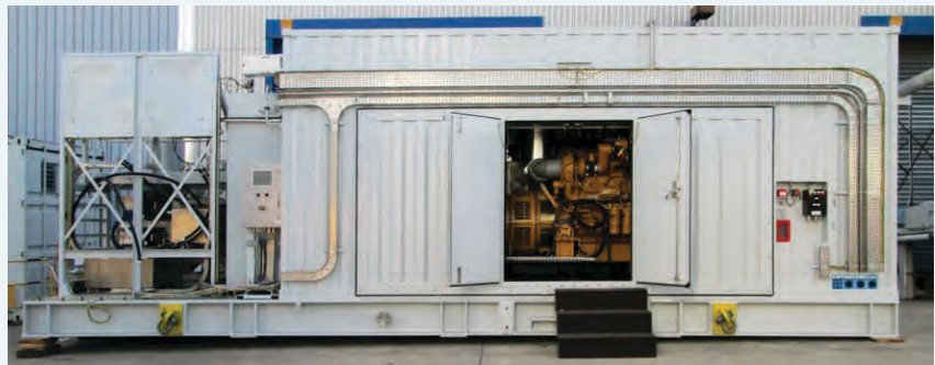
Eneria's power package addressing the strictest TOTAL General and Project Specifications, while being compliant with ATEX/IECEx regulations and DNV GL rules.
