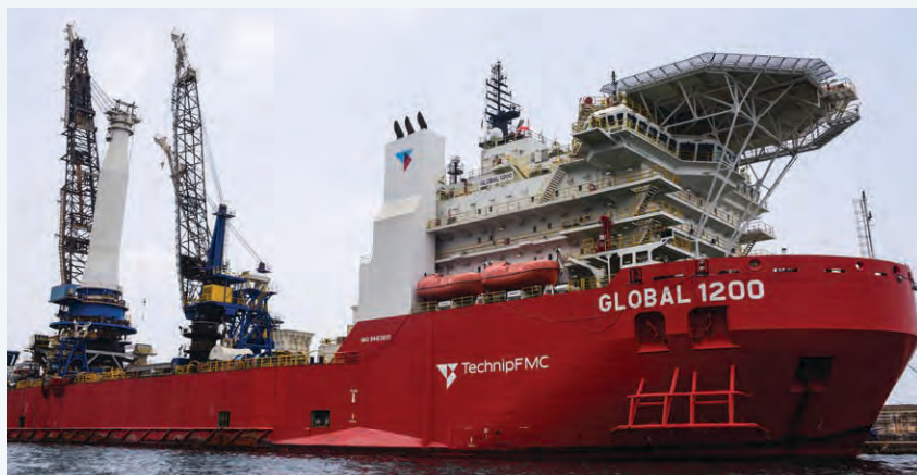
The pipe-laying vessel G1200 performed construction tasks in water depths ranging from just 3 m to 1,200 m and completed an innovative dynamic positioning beach pull operation.
