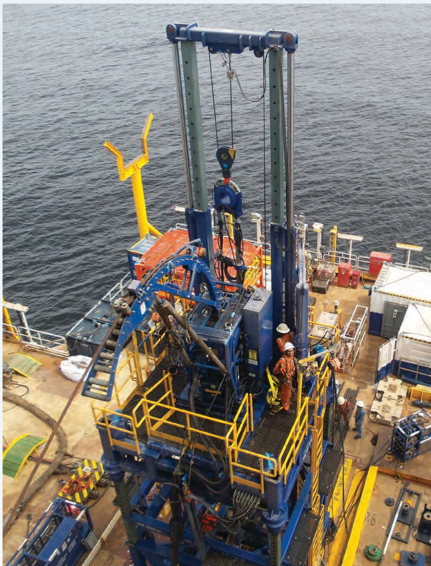
The CT intervention tower, which included the first-time integration of a remotely operated CIRP completion insertion and removal under pressure system, is designed to insert and retrieve long gun strings under wellhead pressure. (Courtesy of Schlumberger)
